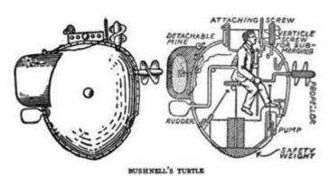
As you can see it was not much of a submarine but it was designed to get up to a British ship and then the detachable mine was left at the ship while Turtle retreated a safe distance. The charge was a timed ignition left secured to the wooden hull of the ship using a drill and ship Auger bit.
